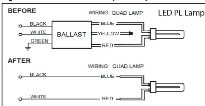
**Figure 2: Retrofit with Two Lamps (GX24q Base)**
